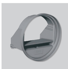
RD BP Low-pressure auto-adjustable flow regulators. (20/100 PA) To be installed inside the duct. 80 mm diameter. Flow rate: 15 or 30 m 3 /h.
